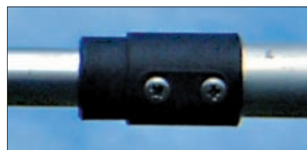
● Fig. 4: Using pre-moulded joining pieces allows adjustments to be made before finally screwing the parts firmly together for permanent use.
