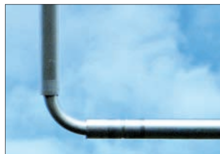
● Fig. 5: These radius-formed bends make the finished design look good as well as giving a sturdy construction.
