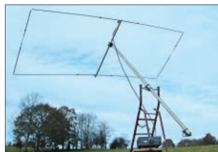
● Fig. 3: Mounted angled upwards at around 45°, the antenna is quite easy to adjust for matching and band centre.
