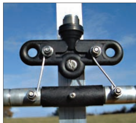
● Fig. 2: A close up of the feed-point arrangement, the two sides of the driven elements are separated and mounted on an insulating g.r.p. strengthener.
